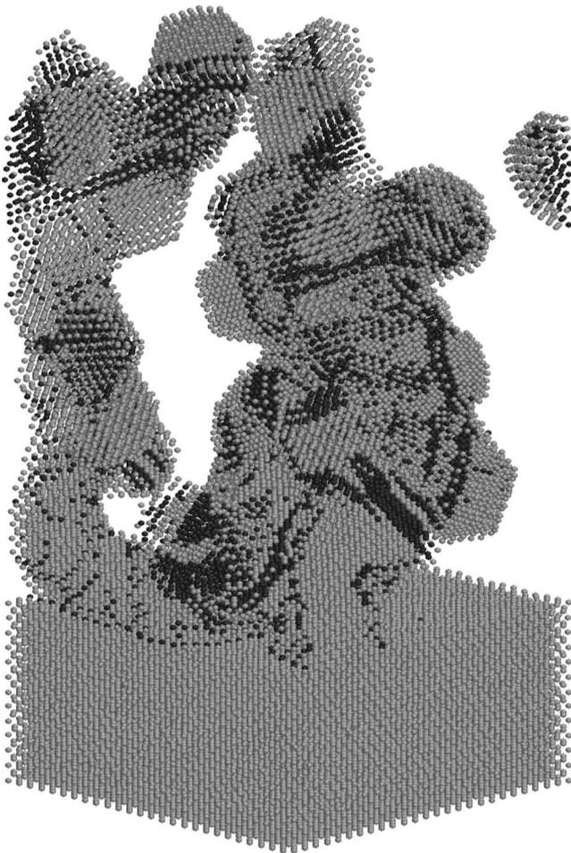
FIG. 2. A snapshot of a typical as-deposited film. Growth appears to be columnar, as clusters easily stick to previously deposited cluster. In some cases, depending on the orientation during impact, clusters can adopt the same crystal directions as the underlying surface, while in most cases the cluster will retain a crystal orientation separate from its surrounding. Atoms in boundaries between different crystal orientations appear slightly darker than atoms in a local fcc configuration.
